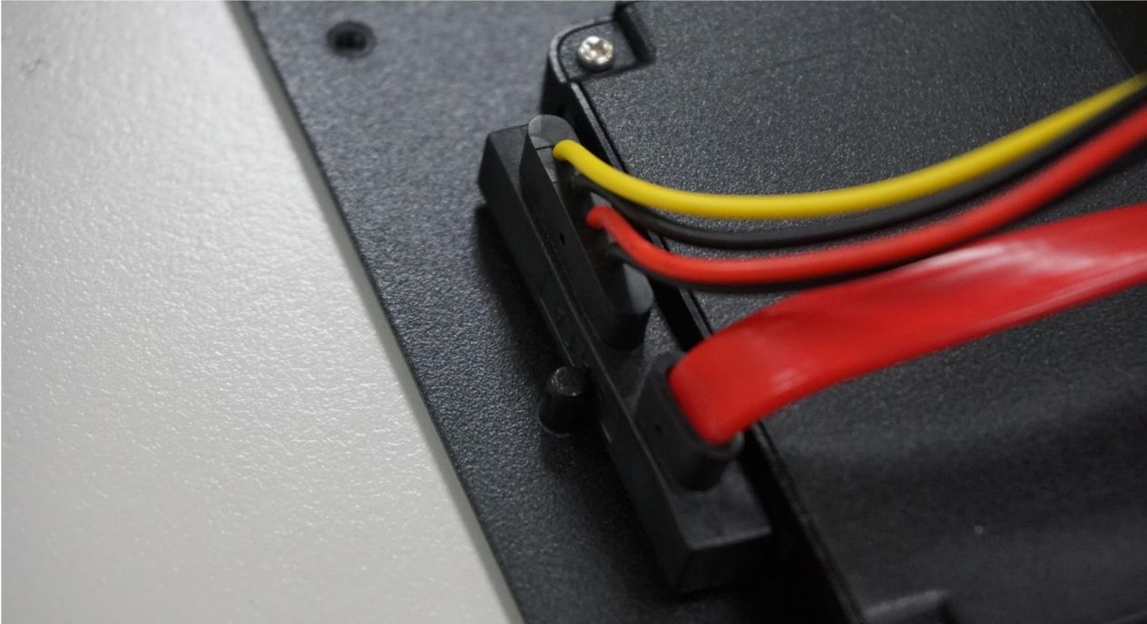
Secure SSD card onto bottom plate with screws (x4) at the side of standoff.
